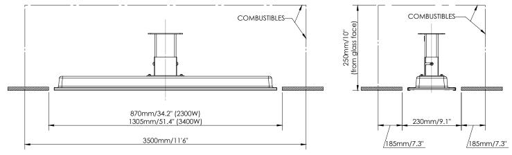
1. Prepare ceiling cut-out with dimensions from images on P.9 to fit ceiling recess frame (a). Heater must be installed with heater surface at least 2400mm above the floor level, with 500mm clearance to the nearest wall on all sides of the heater. Minimum distances to combustibles within cavity must be according to **only one** of the two options shown.
