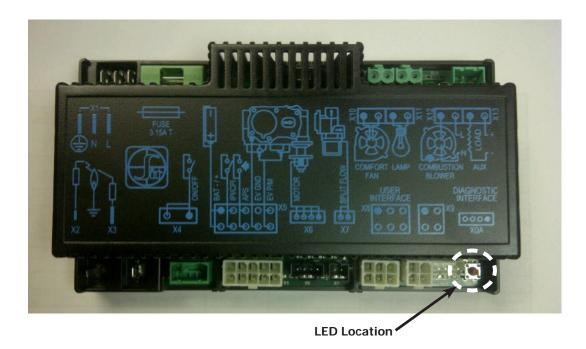
Figure 103: IFC LED Location
