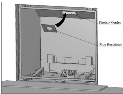
Figure 25: Installation of Flue Restrictor.
