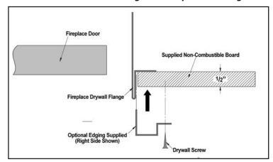
Figure 21. Optional Facing Trim Installation - Right Detail.
