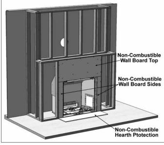
Figure 31: Installation of Wall & Hearth Board.
