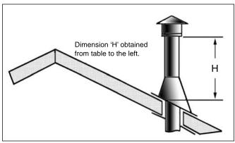
Figure 44: Height of Vertical Termination; Reference Table 5.
