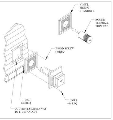
Figure 37: Installation of Vinyl Siding Standoff.
