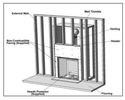
Figure 7. Typical Framing for External Chase - General.
