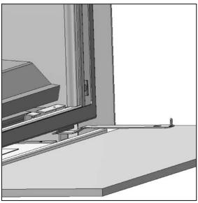
Figure 47: Door Latch Tool in Place.
