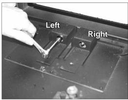
Figure 55: Removing the Gas Orifices.
