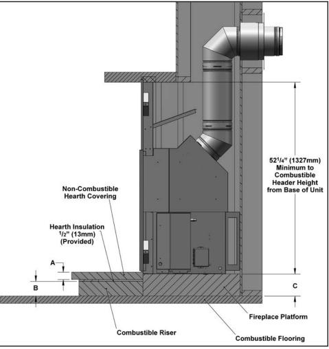
Figure 14. Typical Framing for a Raised Hearth - Detailed.
