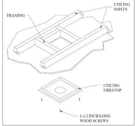
Figure 40: Installation of Ceiling Firestop.
