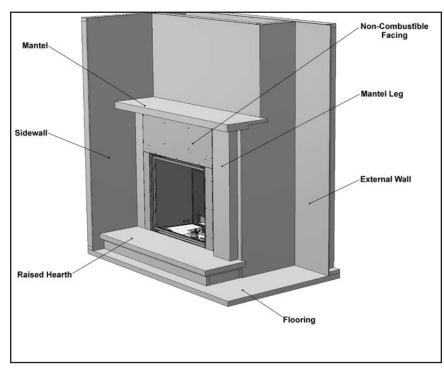
Figure 11. Typical Framing for Sidewalls & Mantel - General.
