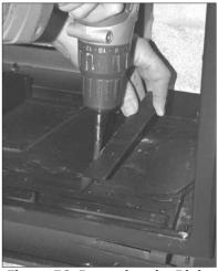
Figure 56: Removing the Right Burner Support.
