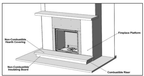
Figure 13. Typical Framing for a Raised Hearth - General.
