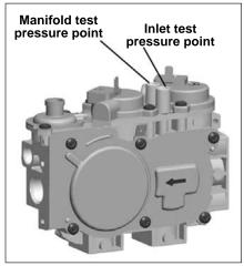
Figure 59: Pressure Test Points.
