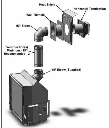
Figure 32: Typical Minimum Vent Configurations
