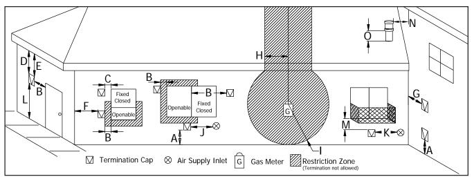
Figure 24. Vent Termination Restrictions, refer to Table 2.
