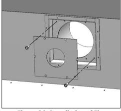
Figure 26: Installation of Flue Restrictor - Close-Up.
