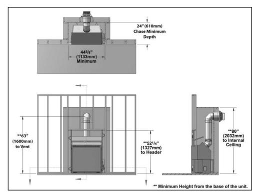
Figure 8. Typical Framing for External Chase - Detailed.
