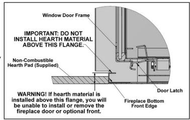
Figure 15. Fireplace Section for a Raised Hearth - WARNING.
