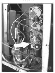
Figure 58: Servo Screws.
