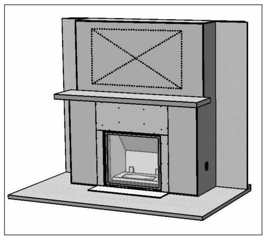
Figure 27: Installation of TV Above the Unit.
