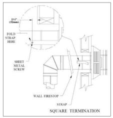
Figure 38: Installation of Vent Pipe to Termination.
