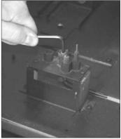
Figure 53: Removing the Pilot Orifice.
