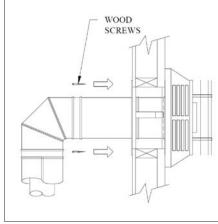
Figure 39: Installation of Wall Fire-stop.
