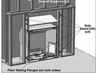
Figure 30: Securing the Unit.
