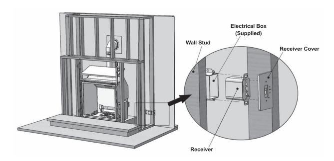
Figure 22. Receiver Installation.
