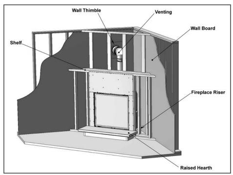
Figure 9. Typical Framing for Corner - General.
