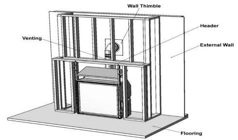
Figure 5. Typical Framing for Internal Chase - General.
