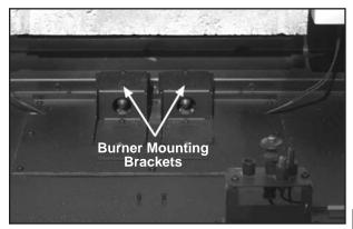
Figure 68: Burner Mounting Brackets.
