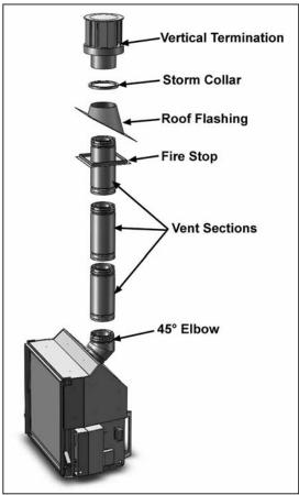
Figure 33: Typical Vent Configurations
