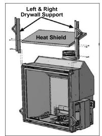
Figure 28: Installation of Supports & Heat shield.
