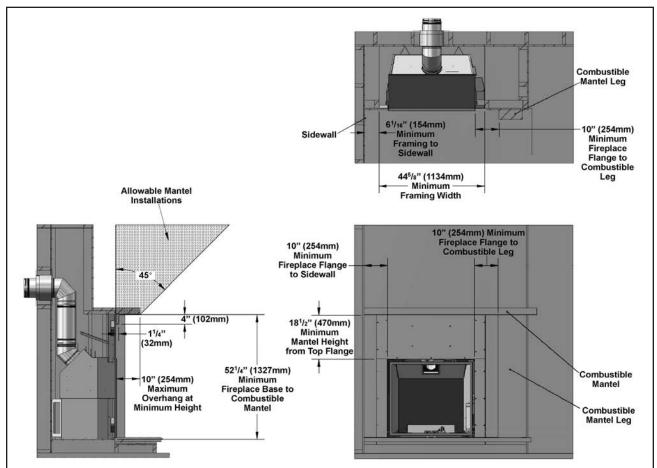
Figure 12. Typical Framing for Sidewalls & Mantel - Detailed.
