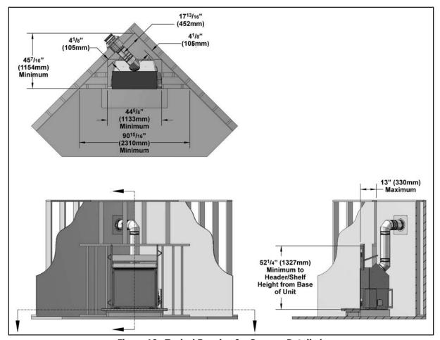
Figure 10. Typical Framing for Corner - Detailed.
