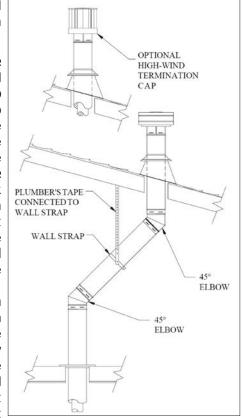
penetrate Figure 41: Vertical Installation using.
