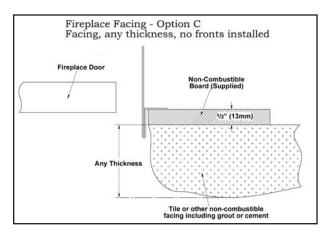
Figure 19. Option 3 - Any Fireplace Facing Without Optional Front Installed.
