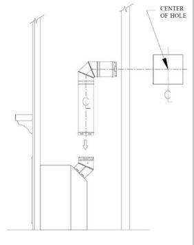
Figure 35: Horizontal Venting and Cut Away.
