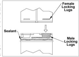
Figure 34: Twist-Lock Connection.
