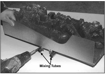
Figure 67: Installing Rear Burner Shield.
