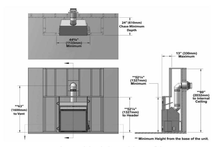
Figure 6. Typical Framing for Internal Chase - Detailed.
