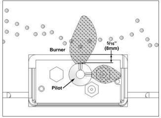
Figure 60: Relationship between ignitor and burner.
