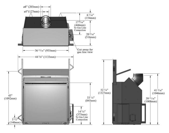
Figure 1. Dimensions of the Firebox.
