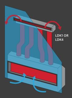
HeatShift naturally delivers up to 125 cubic feet of hot air per minute—without a fan!
