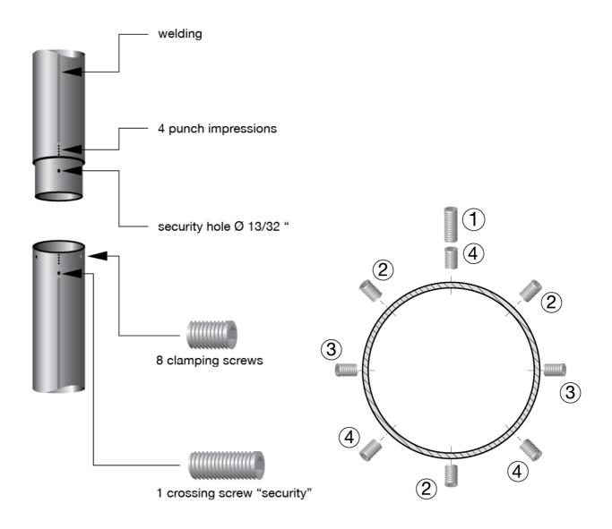
Note: the junction sleeves are provided only when the floor to ceiling height in the room requires several focus pipe in several parts. (you may not find a junction sleeve on 9 feet or less ceiling height)
