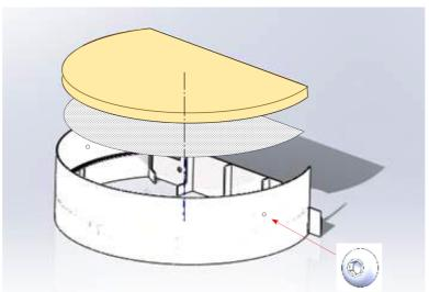
Baseplate must be secured to the fireplace using 2 hexagon bolts.
