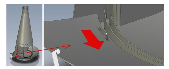
After a few minutes, and making sure the primary fire is well started, add larger wood (between 3 and 7 pieces, depending on their size), directly on top, making sure not to smother the fire. Leave some spaces between the logs for air intake. Adapt the air intake position in order to avoid spillage.
