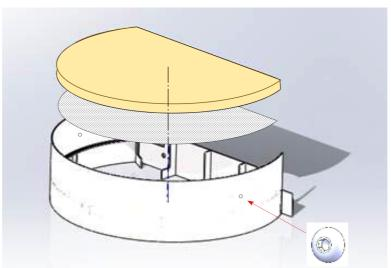
Baseplate must be secured to the fireplace using 2 hexagon headless bolts.
