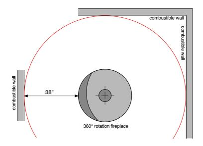
· Wall clearance with optional blocking mechanism:
