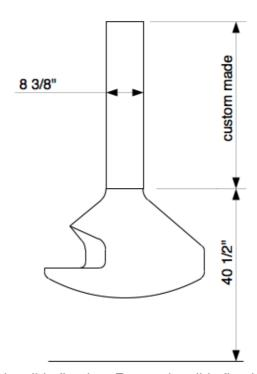
Diagram shows clearance to non-combustible flooring. For combustible flooring, please refer to P.7 diagram.
