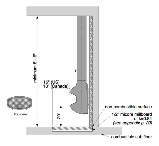
CAUTION: THE DISTANCE TO A COMBUSTIBLE WALL MUST BE MAINTAINED AT 26 inches. PROPERTY DAMAGE OR DEATH CAN OCCUR IF THIS DISTANCE IS NOT MAINTAINED. DRYWALL PRODUCTS LINED WITH PAPER SUCH AS SHEETROCK ARE COMBUSTIBLE. CLEARANCES AS INDICATED FURTHER APPLY.
