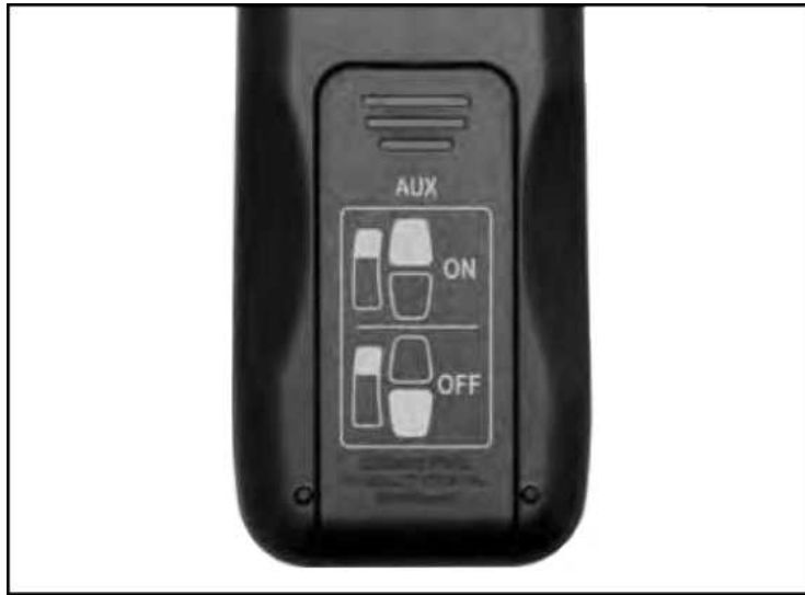
Figure 5: Rear side of hand-held transmitter (battery cover) Instructions for turning the “rear burner” on and off
