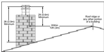
Figure 20: Roof Clearances.
