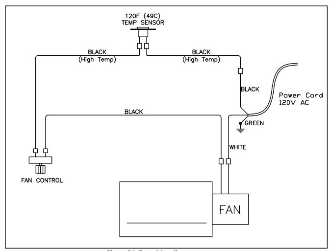
Figure 24: Fan wiring diagram.
