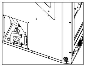
Figure 26: 3/8" NPT Male Pipe Nipple with Cover Removed.
