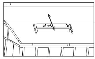
Figure 19: Baffle plate adjustment
