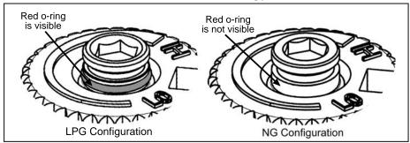
Figure 13: O-ring on valve screw.
