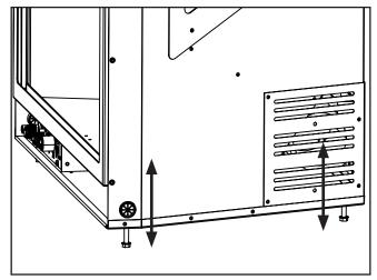
Figure 22: Levelling legs position.
