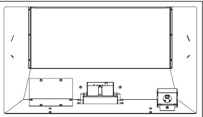
**Figure 41:** Remove the rear porcelain panel by pulling it forward off the ledge.
