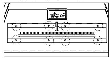
Figure 38: Remove the 8 T20 screws and then remove the bottom panel by lifting up.
