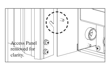
Figure 37: Screw and Hook Close-Up.
