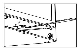
Figure 5: Adjusting the venturi air setting.
