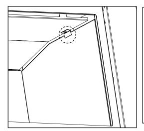
**Figure 40:** Remove the clips which secure the side panels and then pull the bottom of the panels towards the center of the firebox.
