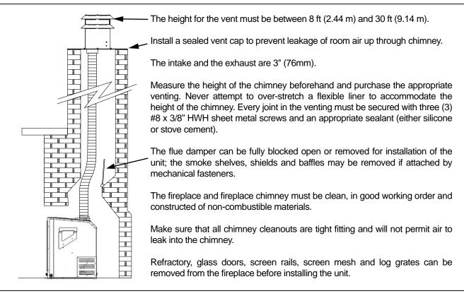
Figure 16: Installation of E30
