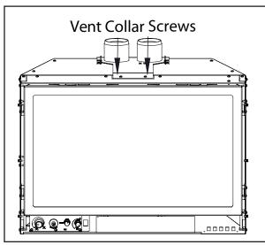
Figure 21: Vent Collar Plate Screw Location.
