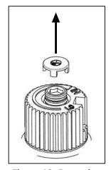
Figure 10: Removing valve cap.
