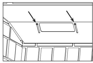
Figure 18: Baffle plate screws
