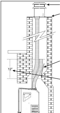
The height for the vent must be between 8 ft (2.44 m) and 30 ft (9.14 m).
