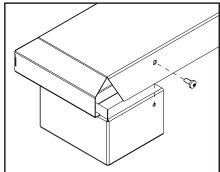
Figure 30b: Installing Base Shelf onto Riser.
