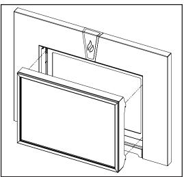
Figure 29b: Installing Safety Screen onto Cabinet Brackets
