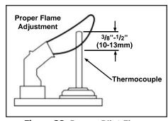
Figure 28: Proper Pilot Flame.
