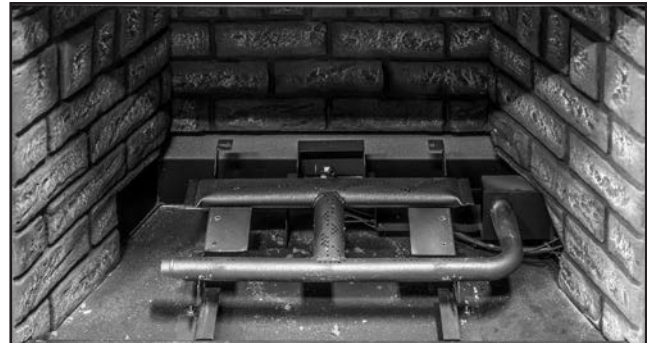
Figure 50: Remove the 6 screws highlighted in figure 49 using a Torx T-20 screwdriver and remove the air deflector
