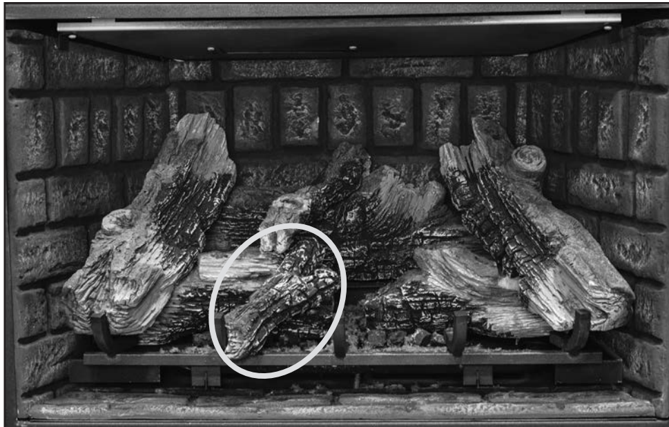
Figure 60: Rest the center top log on top of the left mid log making sure to align the bottom with grate arm.
