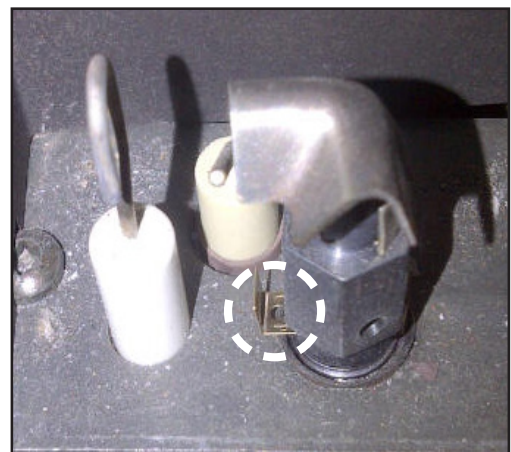
Figure 22. Pilot Slider set to LP
