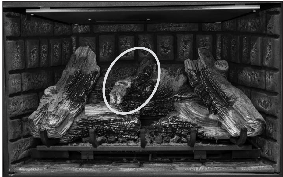
Figure 50: Place the center top crossover log at an angle on top of the rear log and left mid log pins
