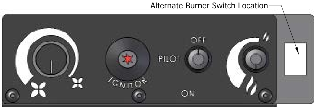
Figure 6: E30 Control Panel.
