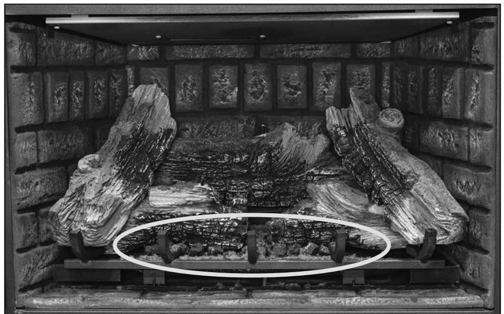
Figure 49: Pull apart Embaglow and spread a thin even layer over the burner area. Brush the ember wool as fine as possible (clump the wool together and separate it using the supplied brush) over the burner tube. Place coals on the air deflector in front of both mid logs as shown. Do Not cover the gaps between the burner and air deflector.
