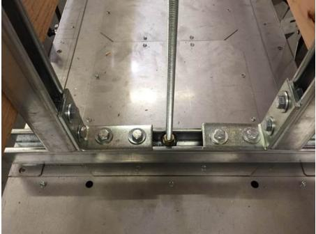
With the brackets and all-thread secure, remove the shipping bracket and check the glass opening height. If it is not correct (20") then loosen the 2 bottom bolts on each vertical piece of Unistrut® and use the all-thread to correct the height (this is why you cut the vertical pieces of Unistrut® short). Once you have the correct height then tighten all the bolts.
