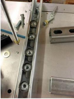
Next you are going to secure a piece of  $1-5/8 \times 1-5/8$ " of Unistrut® to multiple beams in the ceiling. If there is an attic above the beams then secure the Unistrut® on top of the beams, otherwise secure the Unistrut® to the bottom of the beams with the appropriate hardware (not provided).
