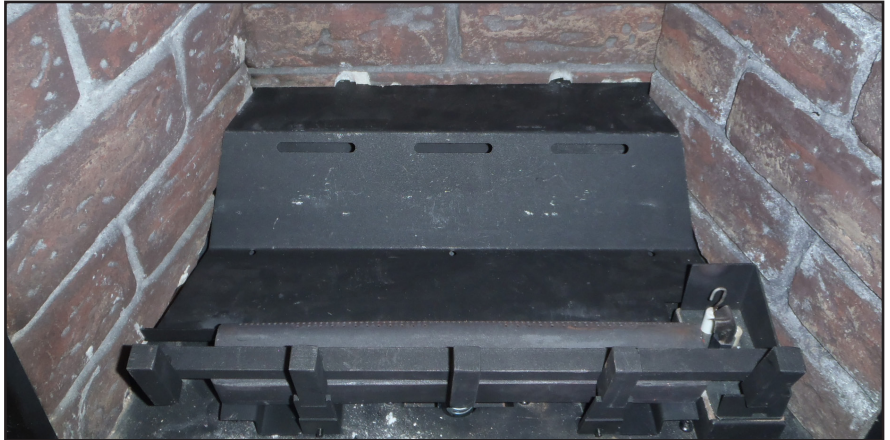
Figure 41. Empty firebox with grate and locator pins.
