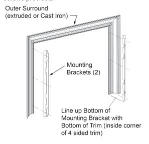
Note: It may be necessary to extend the outer trim to cover the combustible wall opening. Custom non-combustible sheet metal pieces may be added to the extruded aluminum trims and fastened using the screw channel on the back of the trim.
