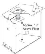
6. Paint liner and gear clamps using black high heat paint (not supplied).
