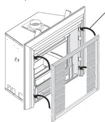
Hook inner front trim onto mounting brackets within outer trim.
