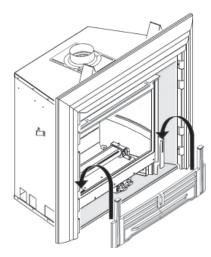
Hook fret onto fret retainer brackets (RA24FK) using RA24DS or FS style fronts
