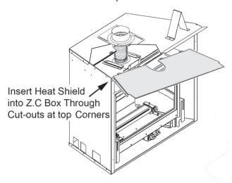
2. Place the tabs at the rear edge of the heat shield into the slots. Secure the heat shield using 2 screws on each side. Screw from within the ZC box.
