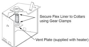
5. Compress or stretch the liner so the vent plate is approximately 19" above the floor.
