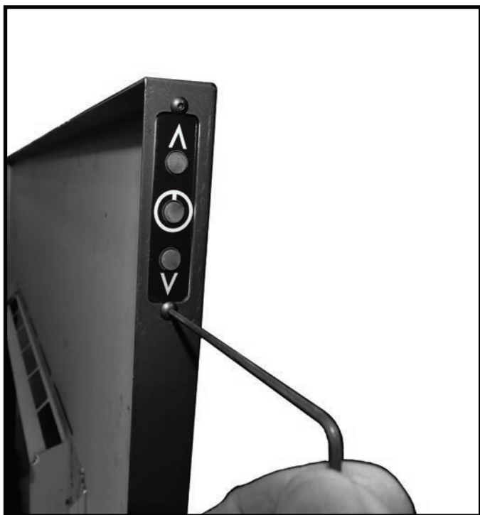
Figure 88: Attaching switch to backing plate.
