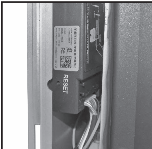
Figure 95: Maxitrol reset button location.
