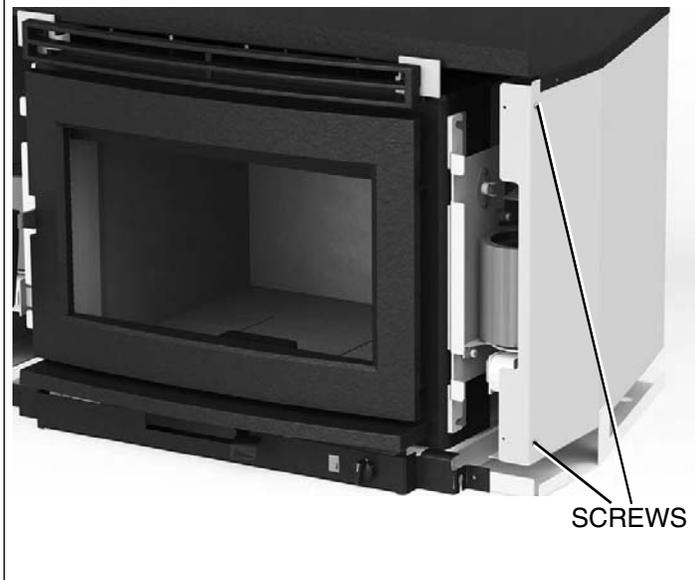
3. With a 3/8" (10mm) wrench, loosen the two bolts securing the blower mounting bracket to the unit. Fig. #3
