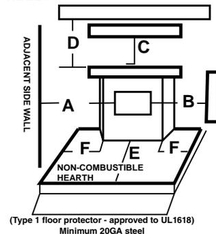
AN ADDITIONAL 1.2 IN/31 MM IN U.S.A. AND 3.2 IN/81 MM IN CANADA OF TYPE 1 FLOOR PROTECTION APPROVED TO UL1618, MINIMUM 20GA STEEL MUST BE USED ADJACENT TO THE HEARTH.// UNE PROTECTION DE PLANCHER DE TYPE 1 APPROUVÉE UL1618, EN ACIER DE 20GA MINIMUM, D'UNE LONGUEUR DE 1.2PO/31MM AUX ÉTATS-UNIS ET 3.2PO/81MM AU CANADA, DOIT PROLONG-
