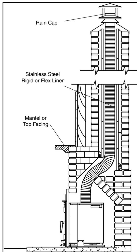
chimney, and will not reduce protection for combustible materials to less than that required by the National Building Code. The Insert must be installed in accordance with local and or national building codes. The two methods of flue connection that are acceptable in most areas are:
